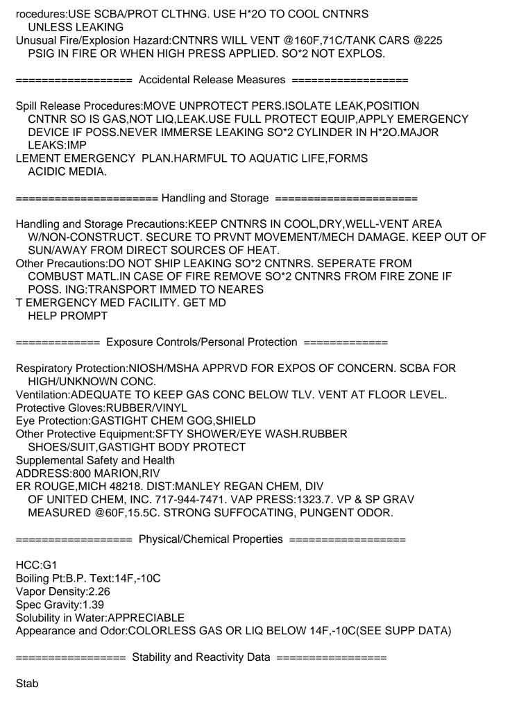
ility Indicator/Materials to Avoid:YES STRONG ALKALIES,OXIDIZING AGENTS. MOIST GAS CORRODES METALS. Stability Condition to Avoid:PRESENCE OF MOISTURE & HIGH TEMPS. STORAGE IN CONFINED SPACE
