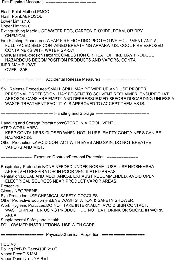
Boiling Pt:B.P. Text:410F,210C Vapor Pres: O.5 MM Vapor Density:>1.0 AIR=1 Spec Gra
