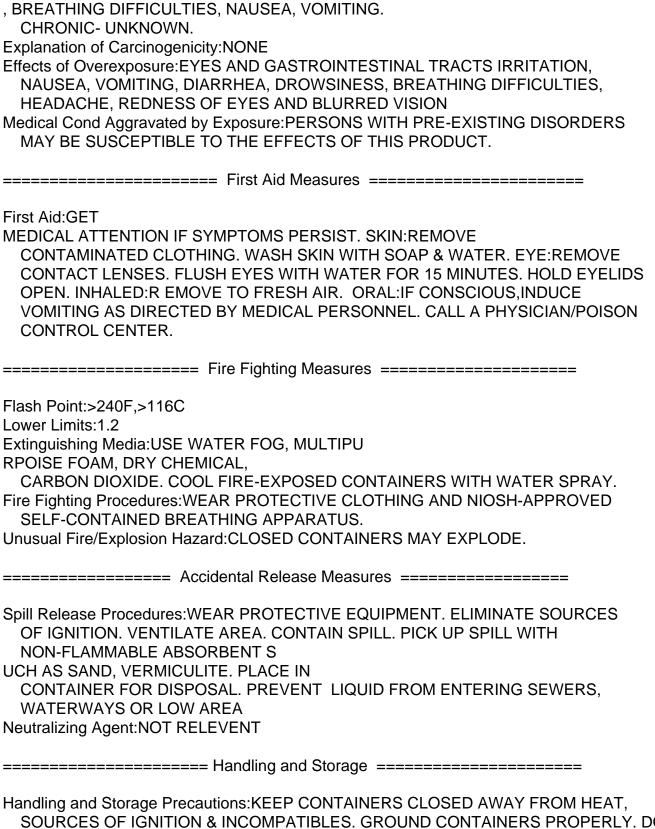
SOURCES OF IGNITION & INCOMPATIBLES. GROUND CONTAINERS PROPERLY. DO NOT STORE IN CONTAINERS OF AL, CU OR ZINC.
