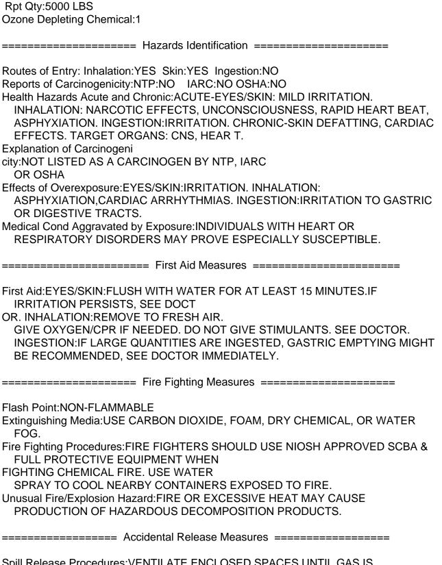
Spill Release Procedures: VENTILATE ENCLOSED SPACES UNTIL GAS IS DISPERSED. USE RESPIRATOR AND PROTECTIVE CLOTHING. ABSORB IN INERT MATERIAL AND PLACE IN APPROPIATE DISPOSAL CONTAINER AND SEAL. FLUSH AREA WITH LARGE A
