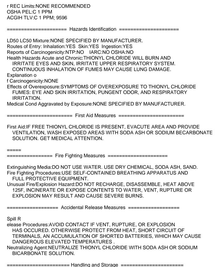
Handling and Storage Precautions: DO NOT SHORT CIRCUIT, HEAT ABOVE 125C
